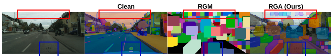
Fig. 7. Visualization of Region-Guided Attack (RGA) on SAM under different region types. The background (e.g., sky) is misled to be fragmented into small regions, while small foreground objects are expanded into abnormally large regions. This demonstrates RGA's capability to selectively disrupt the segmentation of different region types in a targeted manner.
