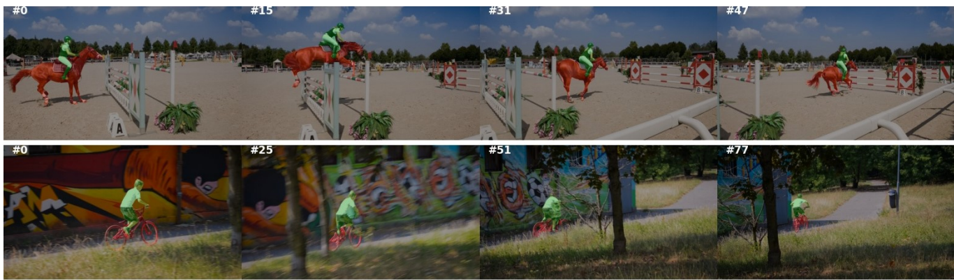
Fig. 8. Visualization of representative segmentation results on DAVIS2017. Ground truth is shown in the first frame and predicted results are shown in the following frames. We want to emphasize that SRF uses only bounding boxes but not masks in initialization, and SRF has produced quite satisfactory results. Best viewed in color with zoom-in.
