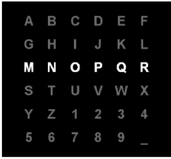
Fig. 1. Stimulus matrix of the P300 speller diagram
